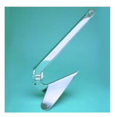
The plow (or CQR) anchor is a burying anchor that has a hinged shank to keep it from breaking out if the boat swings to one side. I would use the plow as a primary working anchor. It holds well under large loads and in most bottoms, although it can be difficult to set in grass or weeds. It can be stored on the bow. The Delta is similar to a CQR, but its shank is one piece. It also holds well in most bottoms, other than large rocks and weeds, and can be stored on the bow.
