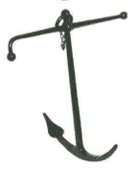
A traditional anchor with relatively small flukes perpendicular to the stock and connected by a shank.
