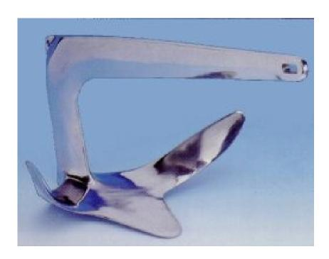
Very popular with cruisers, the tri-point has no moving parts to get jammed or that give, works with a variety of bottoms, and easily plows into softer surfaces. It features three round-edged flukes that curl out from the dogleg shank. It was invented in Scotland to secure floating oil rigs, so you know it's strong. The tri-point has high holding power and low breakout force.
